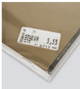
Figure 12 Pressure sensitive adhesives are one of the main applications of hot melts.
